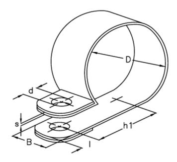
$\begin{array}{ll} d & = 8.4 \\ \text{Diameter D} = 17 \\ \text{h1} & = 21.0 \\ \text{I} & = 8.5 \\ \text{s} & = 0.8 \\ \text{Width B} & = 20 \\ \end{array}$
